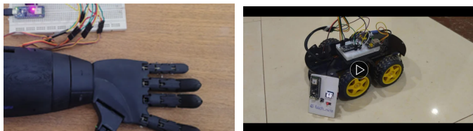
Fig. 4: Left: the voice activated robotic hand from a student team in Brazil [9]. Right: the gesture controlled RC car from a student team in Kenya [10].
